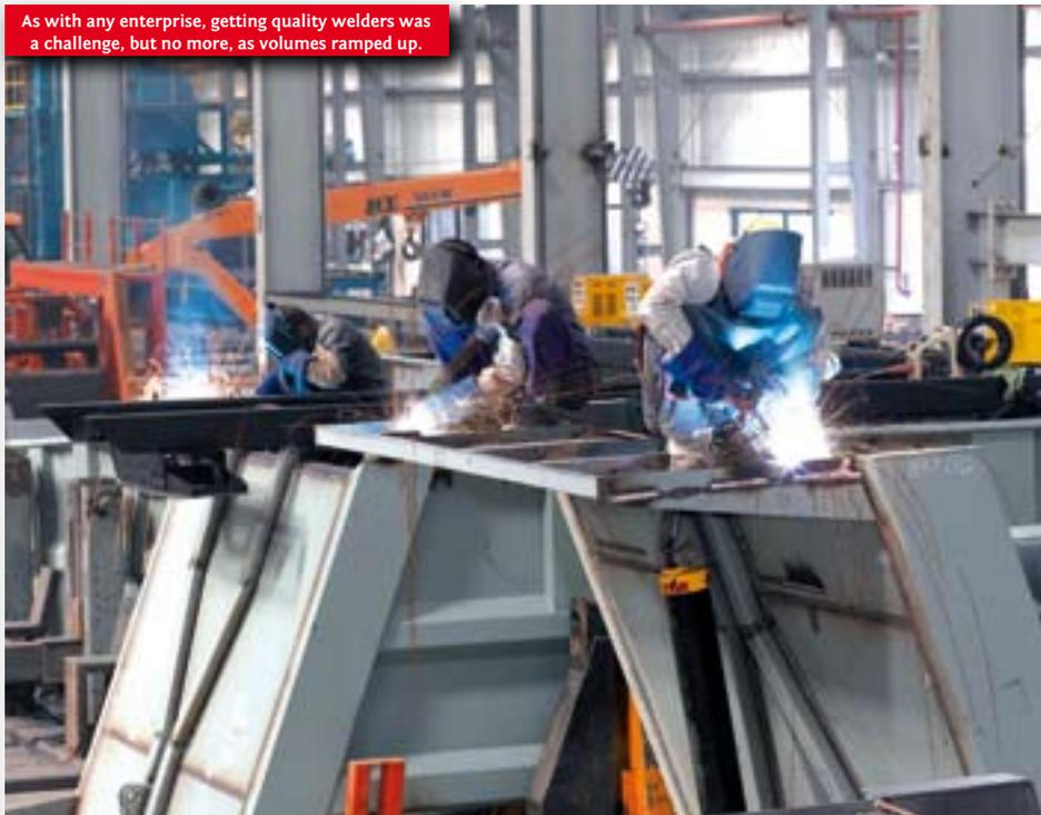
cubing stations. At this juncture, the now complete tipper body is welded to the chassis, from where it goes to the paint shop. In this manner, AMW can roll out a fully built vehicle in hours, where other OEMs may
